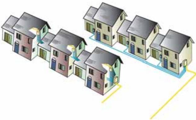
A significant majority of new condominiums and town homes are constructed using a horizontal layout that very closely resembles the arrangement of single family homes. Because of the similarity of single family homes the FTTP connector scheme is often identically equivalent. Usually the network interface will be a Fiber Distribution Terminal located on the exterior surface of the structure.
